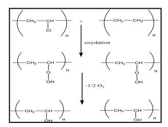
Figure 2.a: thermal degradation of PVC / HDPE and training hydroxide OH.
