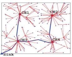
Fig : The hybrid CS data collection method in cluster structure[1]
