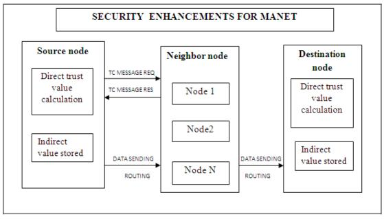
Figure1. Architecture diagram for Security Enhancement for MANET
