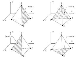
Fig.1. Different faces of a tetrahedron element
