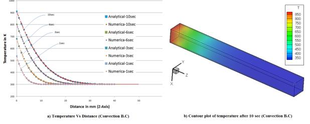
Fig.5. Temperature Vs Distance and contour plot of temperature after 10sec (Convection B.C)
