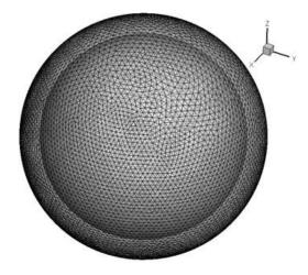
Fig.8. Computational domain of Sphere
