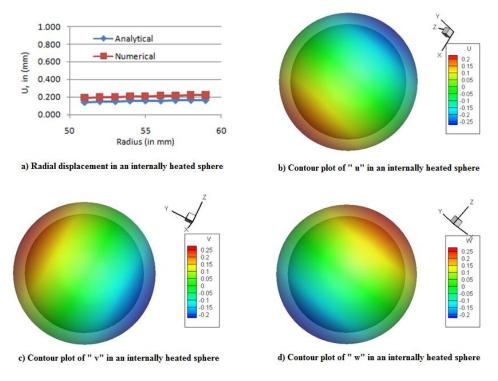
Fig.9. Radial displacement and Contour plots of u, v and w in an internally heated sphere.
