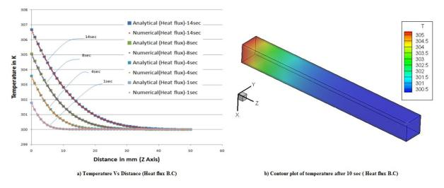
Fig.4. Temperature Vs Distance and contour plot of temperature after 10sec (Heat flux B.C)
