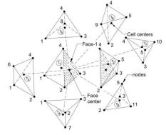
Fig.2. Cell center values used for the evaluation of the gradient trough faces
