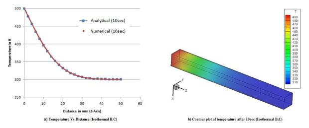
Fig.6. Temperature Vs Distance and contour plot of temperature after 10sec (Isothermal B.C)
