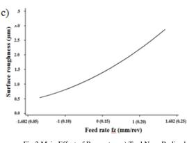
Fig 2 Main Effect of Parameters a) Tool Nose Radius b) Cutting Speed c) Feed Rate
