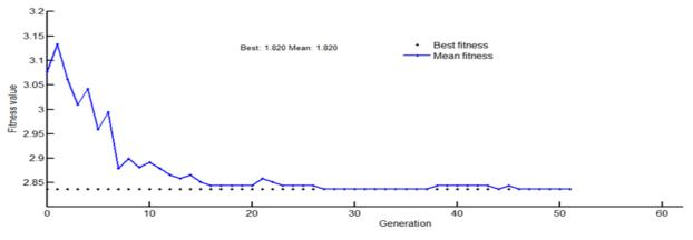
Figure 7 Optimization of Surface Roughness with Subsequent Generations
