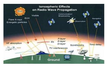
Fig 1: Ionospheric Effects on Radio Wave Propagation
