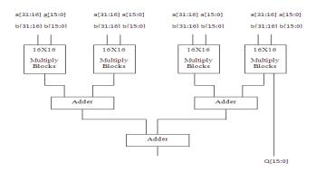
Figure 3: 32X32 Bits proposed Vedic Multiplier
