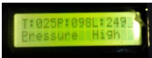
Fig 8. Pressure high alarm (More load)
