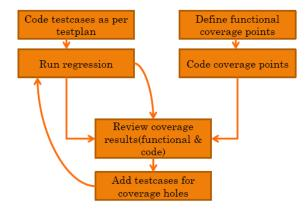
Fig. 2. Coverage Driven Verification Flow
