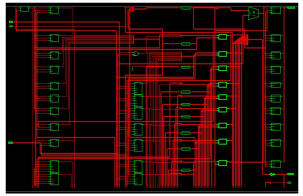
Fig. 8 RTL View of Non Restoring Division Algorithm.
