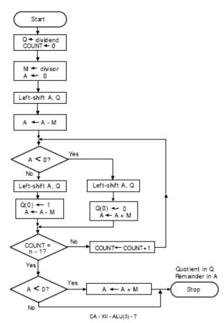
Fig. 3 Flowchart of Restoring Division Algorithm.
