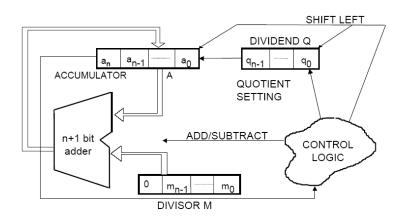
Fig. 1 Hardware Design of Restoring Division Algorithm.
