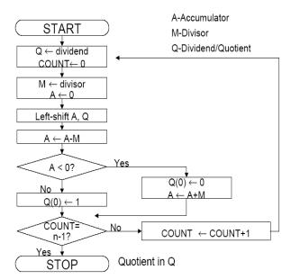
Fig. 2 Flow chart of Restoring Division Algorithm.
