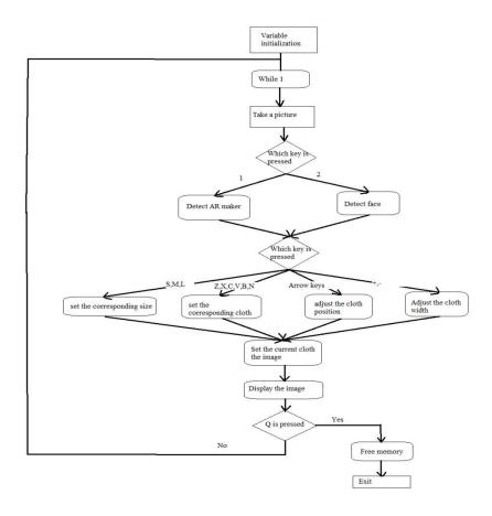
Fig 3. Flow Chart for Virtual Fitting Room
