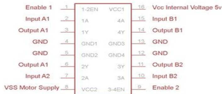
Fig 3.Pinout of L293D
