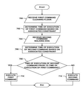
Figure 4 Flow Charts for robotic unit
