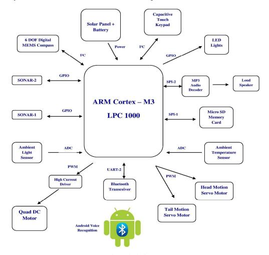
Fig 2 Block diagram
