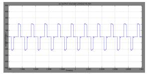
Fig 3 Alternating Voltage Obtained from FBTL Converter Fig 3 shows the output waveform obtained from the inverter when a 250V DC input voltage is fed to it. The switches conduct providing two operation modes as mentioned above and due to the conduction of the switches losses occur. And also the stress in the voltage is been produced. For a 250V input DC voltage the inverted output from a FBTL converter is about 200V. This is only due to the conduction loss and voltage stress.
