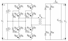
Fig 1 Full Bridge Three Level DC-DC Converter
