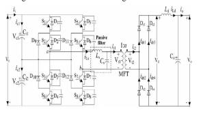
Fig 2 Circuit Diagram For Improved ZVS Full Bridge Three Level Dc-Dc Converter
