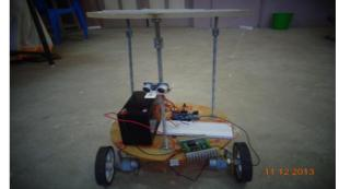
Fig. 7 Object detection and avoidance by using Ultrasonic sensor
