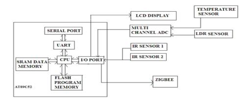
**FIGURE 3.1 Block Diagram Of Transmitter**
