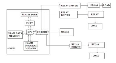
3.2 FIGURE Block Diagram Of Receiver
